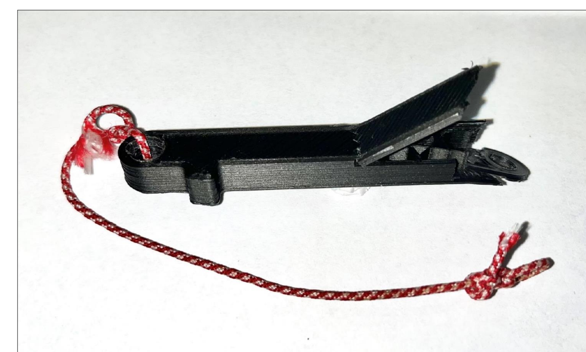
Short Arms V.1 made of PLA. Strapped vertically, this was able to hold at least 11 kg.
